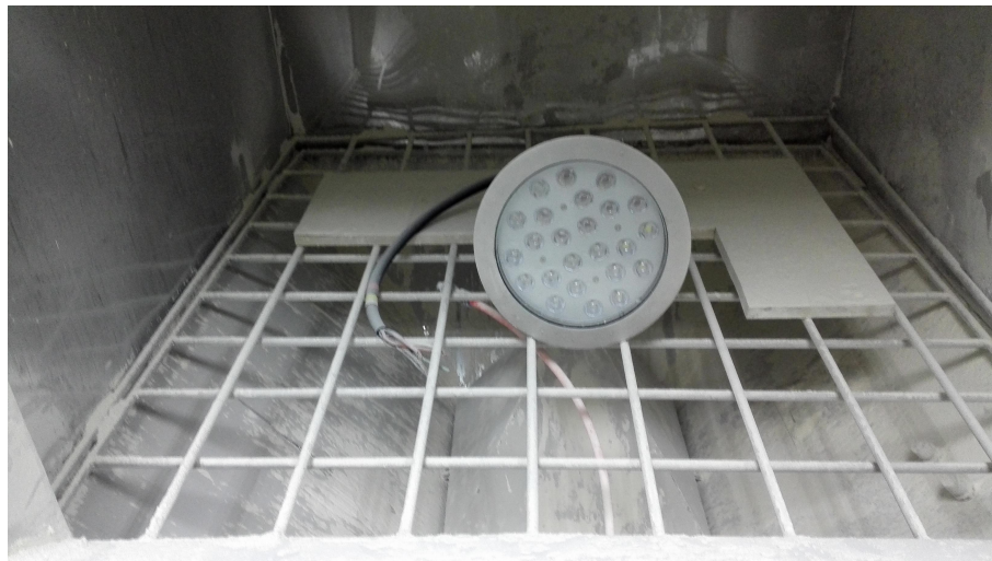
Photo 2: IP6X test of model RS-UW96W316X
