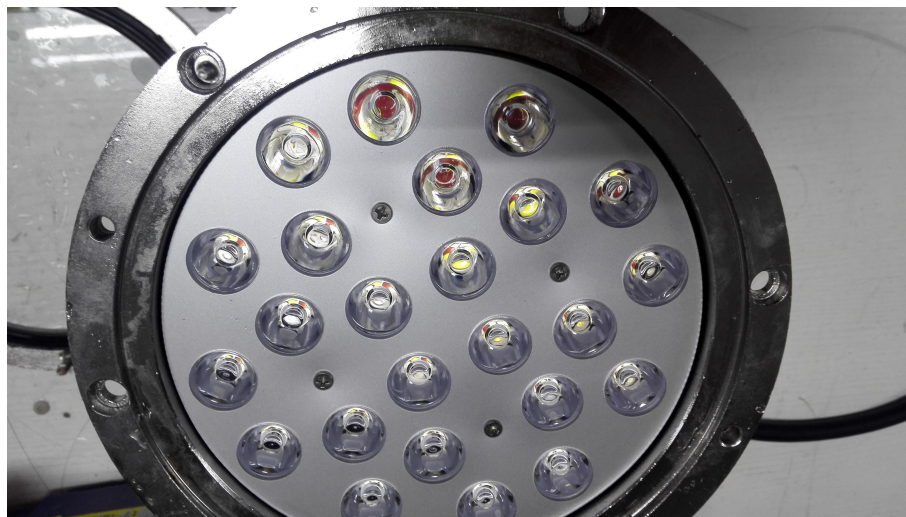
Photo 4: Test result after IP6X and IPX8 test
