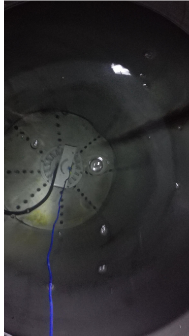
Photo 3: IPX8 test of model RS-UW96W316X
